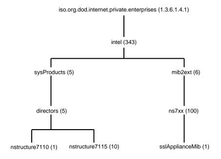
Figure 6-1: Intel's MIB Tree (top level)
